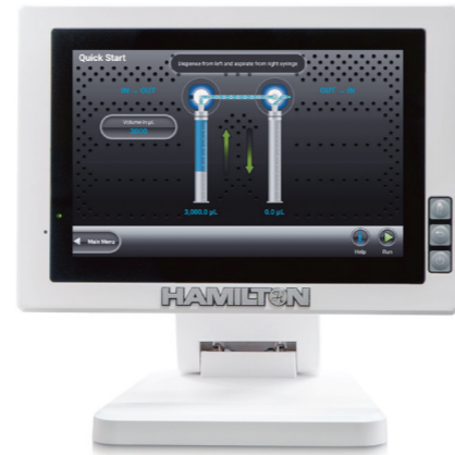
Continuous Dispenser One syringe fills while the other syringe is dispensing from the same reservoir.
