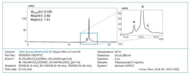
Smaller column IDs that allow lower flow rates and volatile mobile phases are necessities for coupling to mass detection. Such high sensitivity analyses are ideally performed using YMC Accura BioPro IEX columns. Another positive effect is the decreased solvent consumption and lower amount of sample required.
