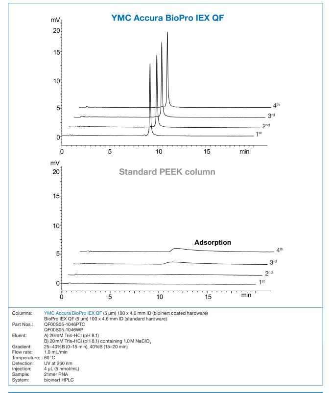
Oligonucleotides generally exhibit poor peak shape and therefore low recovery in AEX analysis, mainly due to adsorption onto the column hardware. YMC Accura BioPro IEX columns provide high recovery and very good peak shapes from the first injection. This makes YMC Accura BioPro IEX QF columns ideal for the analysis of oligonucleotides with reproducible results. The columns show stable peak areas from the 1<sup>st</sup> injection, so that no preconditioning is required.
