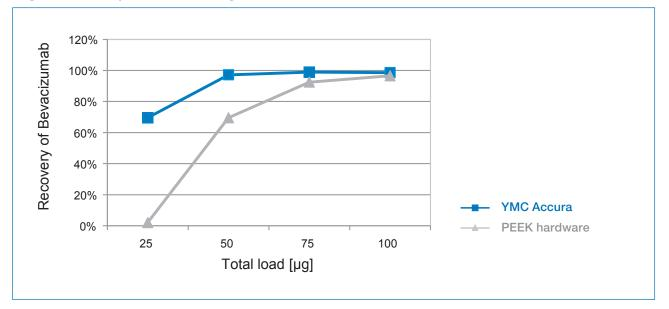
The high inertness of YMC Accura BioPro IEX columns also requires no preconditioning in CEX analyses. Especially at low loading amounts, YMC Accura BioPro IEX SF columns provide higher recoveries compared to the standard PEEK column.
