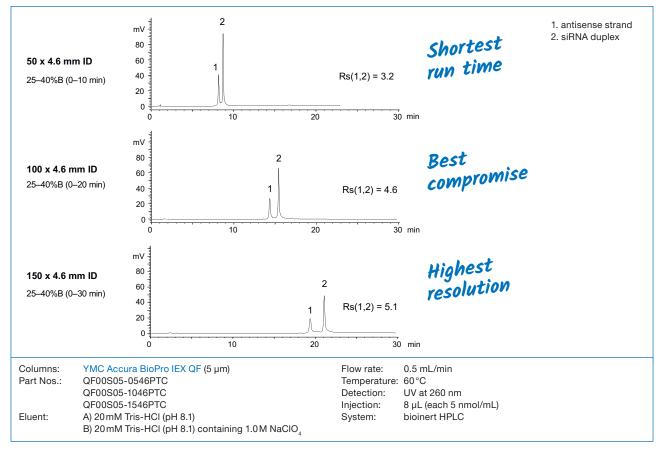
YMC Accura BioPro IEX columns are available with different lengths for specific purposes. Short columns provide short run times and high throughput, whilst retaining good resolution. Longer columns offer a higher resolution that is required for challenging samples, such as the separation of single- and double-stranded RNA.
