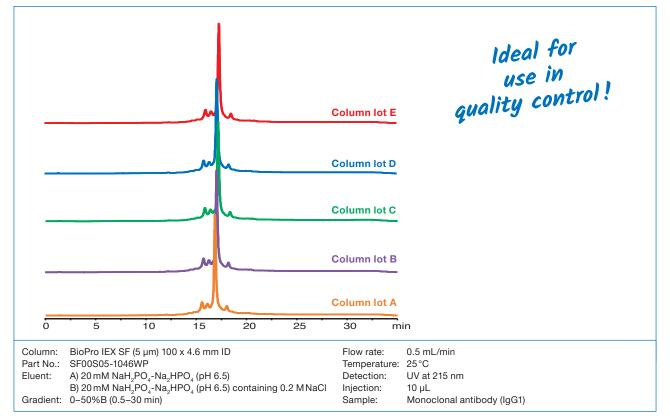
BioPro IEX columns exhibit excellent batch-to-batch reproducibility – as in this example – for mAb analysis with resolution of peaks for small charge variants. All gel batches are inspected by rigorous quality control tests and must meet the required criteria before release.
