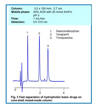
Presence of a basic group on the surface also allows to retain corresponding acidic counter-ion (Fig. 4) The method can be extended for analysis of other acidic counter-ions and corresponding hydrophobic drugs. Mixed-mode core-shell columns showed excellent selectivity towards separation of isomers. Two organic acids, 3-mitrophthalic and 4-nitrophtalic acids were separated on Coresep SB column (Fig. 5).
