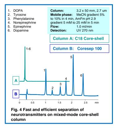
columns as their low hydrophobicity is not enough to provide sufficient retention. The dual synergistic mechanisms of mixed-mode chromatography combined with the core-shell particle allow retention and separation of these 5 compounds within a one minute run time.
